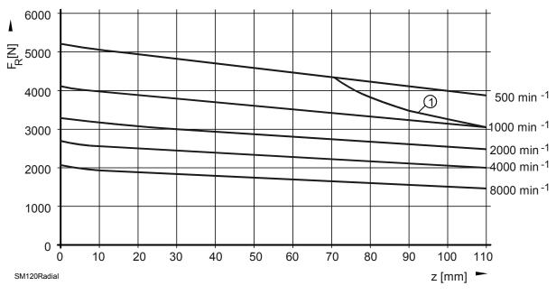
Figure 7-90, SM 120A - Permissible Radial Force on the Motor Shaft
