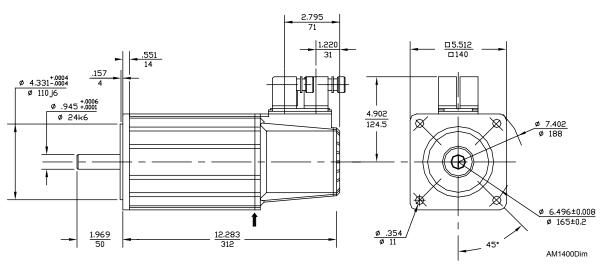
Figure 7-43, AM 1400 Series - Dimensional Drawing
