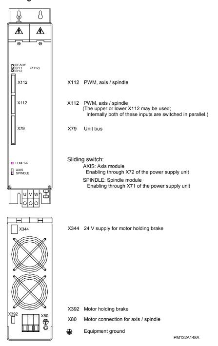
Figure 6-10, PM 132A and PM 148A Power Module, Connections
