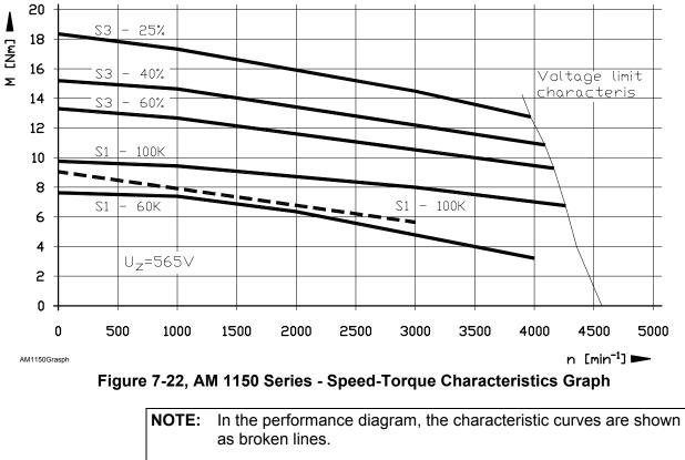
The diagram shows the characteristic curves as determined on a test stand for one motor mounted without thermal insulation.
