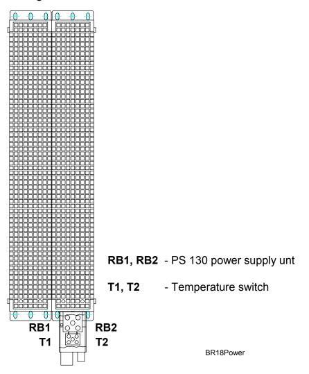
Figure 6-20, BR 18 Braking Resistor Module, Connections
