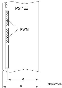
Figure 2-1, Module Width Measures
