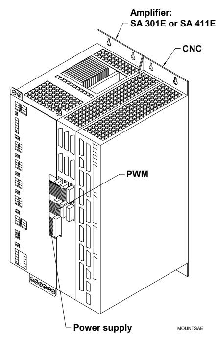
Figure 5-18, Mounting the SA 301E, SA 411E Amplifier
