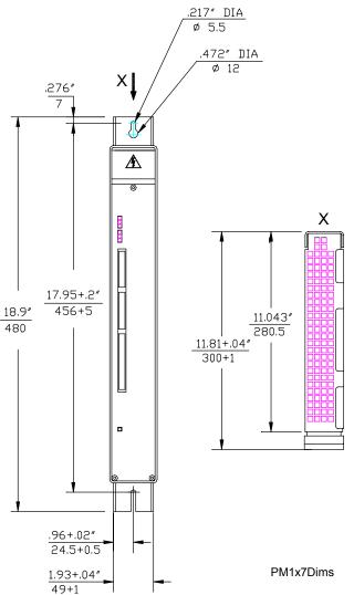
Figure 6-34, PM 107, PM 207 Power Module, Dimensions
