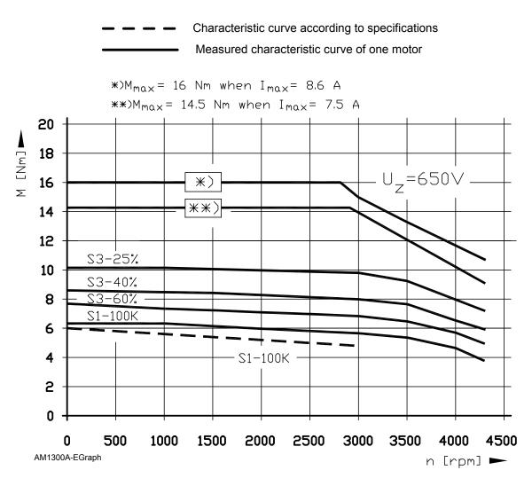
Figure 7-26, AM 1300A–E Series - Speed-Torque Characteristics Graph
