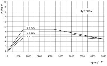
Figure 7-47, SM 055A - Power Characteristics Graph
