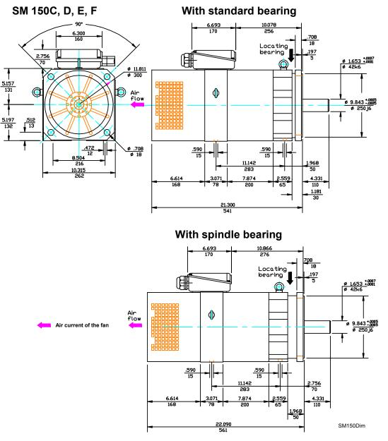
Figure 7-75, SM 150C–F - Dimensional Drawing
