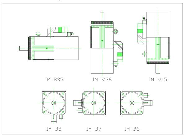
Figure 7-9, Design B35 - Mounting Flange Configurations
