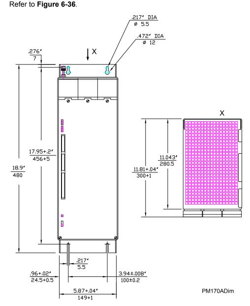
Figure 6-36, PM 170A Power Module, Dimensions
