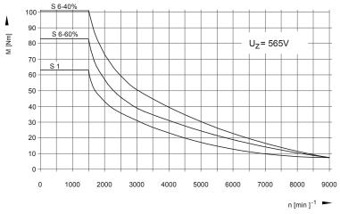
Figure 7-52, SM 100A Torque Characteristics Graph
