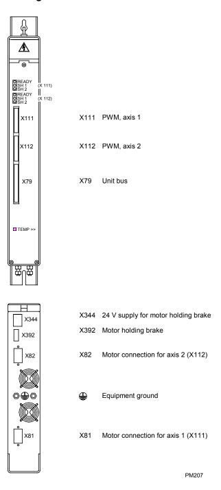
Figure 6-14, PM 207 Power Module, Connections
