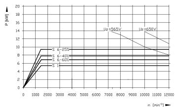
Figure 7-55, SM 055C–F - Power Characteristics Graph SM 055C–F - Torque Characteristics Graph
