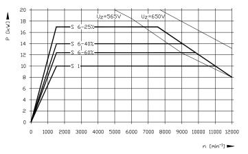
Figure 7-59, SM 100C-F - Power Characteristics Graph
