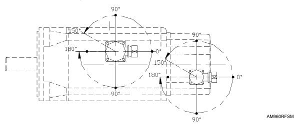
Figure 7-14, AM 960, AM 1160 Series (starting in mid-2002) Rotatable Flange Socket
