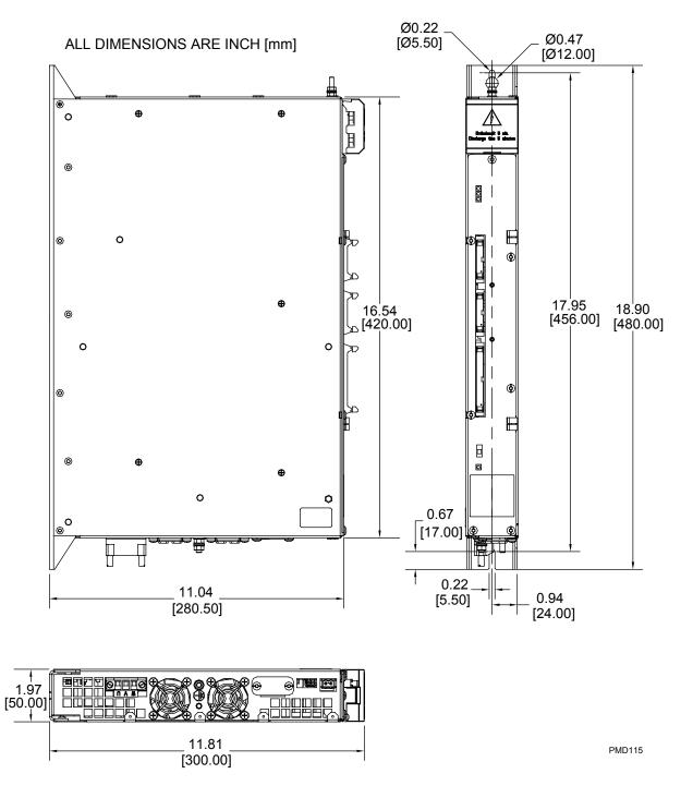
Figure 6-38, PMD 115 Power Module, Dimensions
