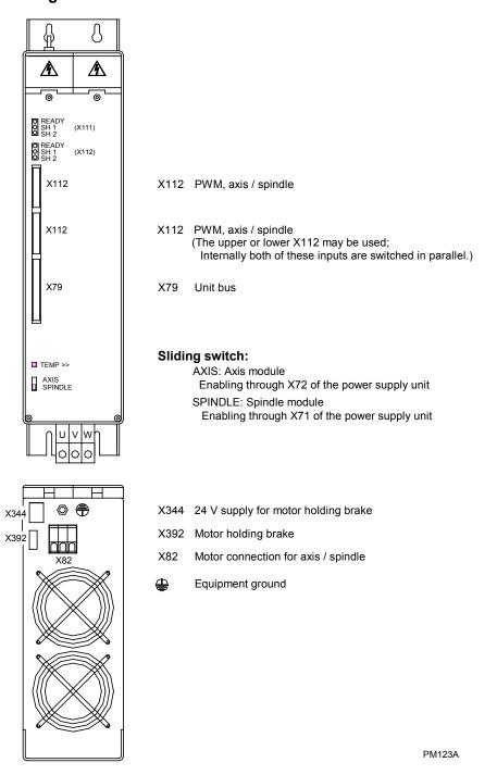
Figure 6-8, PM 123A Power Module, Connections
