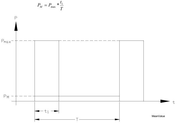
Figure 3-1, Mean Value of Braking Performance Example
