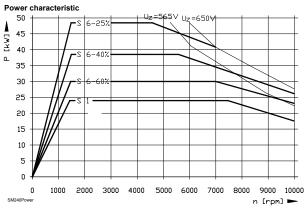
Figure 7-67, SM 240C-F - Power Characteristics Graph
