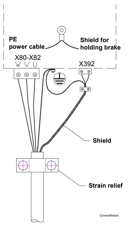
Figure 6-25, Connecting the Motors
