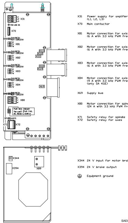
Motor connection for axis 1 (to X111) (6 A with 3.3 kHz PWM frequency) Motor connection for axis 2 (to X112) (6 A with 3.3 kHz PWM frequency) Motor connection for axis 3 (to X113) (6 A with 3.3 kHz PWM frequency)
