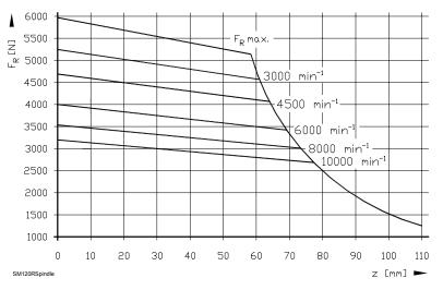
Figure 7-98, SM 150D, SM 150F, SM 200D, SM 200F, SM 240D, SM 240F - with Spindle Bearing - Permissible Radial Force on the Motor Shaft
