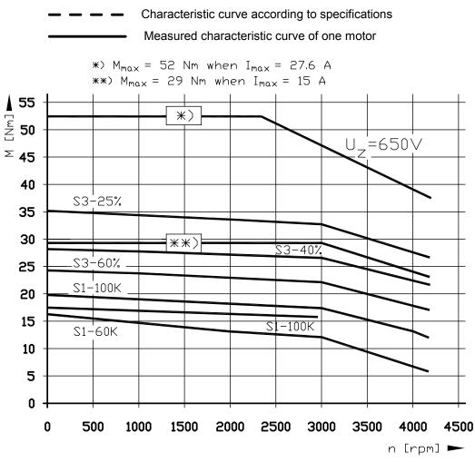
Figure 7-34, AM 1550C-E Series - Speed-Torque Characteristics Graph
