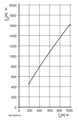
Figure 7-84, AM 1550 Series - Permissible Axial Force on the Motor Shaft (F<sub>A2</sub>)
