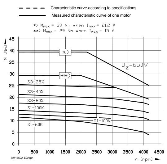
Figure 7-33, AM 1550A–E Series - Speed-Torque Characteristics Graph
