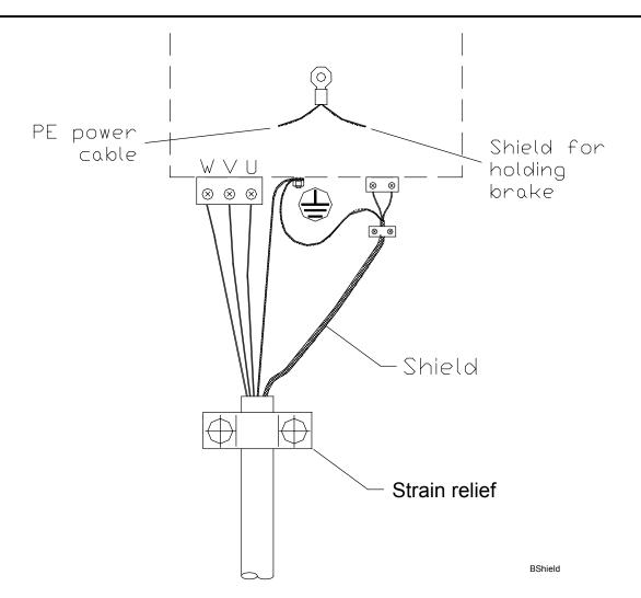
Figure 7-8, Shield for Holding Brake Installation
