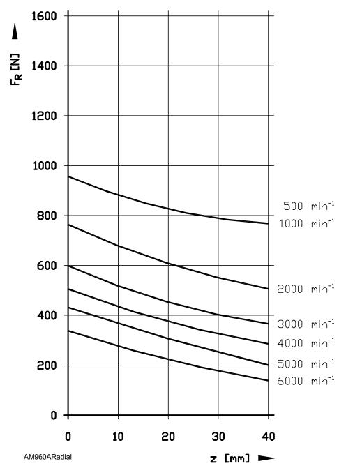
Figure 7-80, AM 960A, AM 960AB - Maximum Permissible Radial Force (F<sub>Rmax</sub>)
