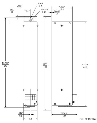
Figure 5-28, BR 10F and BR 18F Braking Resistor Dimensions
