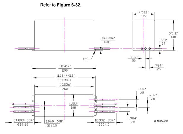
Figure 6-32, LF 180A Line Filter, Dimensions
