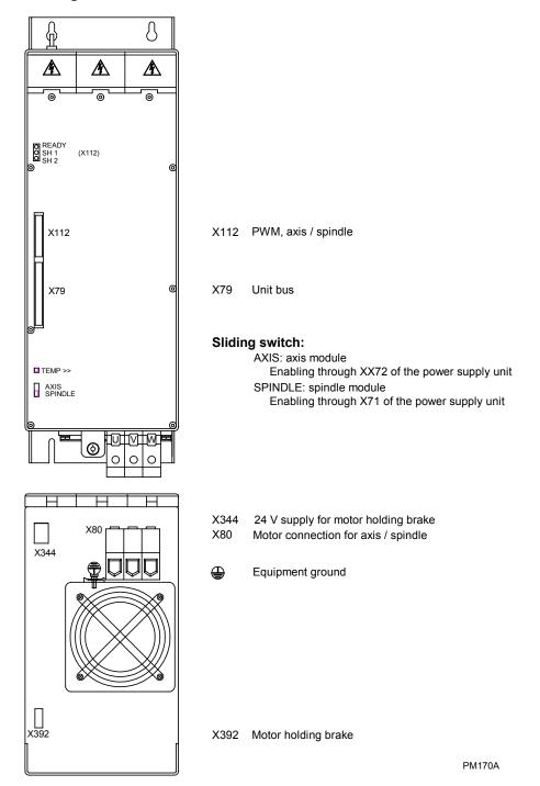
Figure 6-12, PM 170A Power Module, Connections
