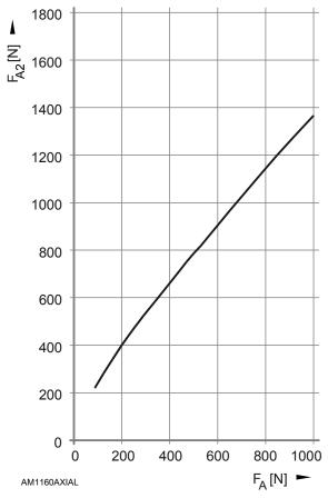
Figure 7-82, AM 1160 Series - Permissible Axial Force on the Motor Shaft (F<sub>A2</sub>)
