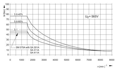
Figure 7-50, SM 075A Torque Characteristics Graph
