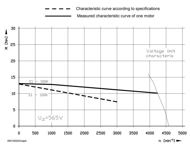
Figure 7-28, AM 1400A Series - Speed-Torque Characteristics Graph (n<sub>N</sub>=3000 rpm)
