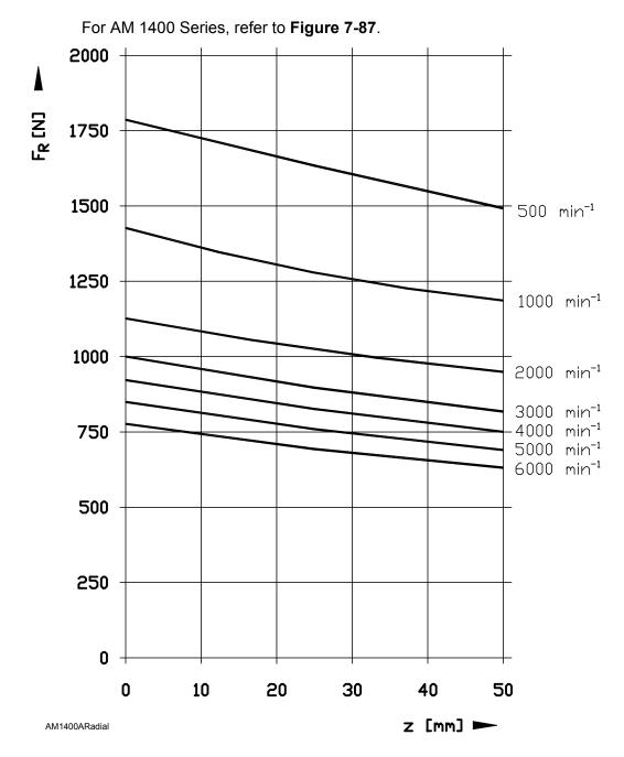
Figure 7-87, AM 1400 Series - Permissible Radial Force on the Motor Shaft (F<sub>R</sub>)
