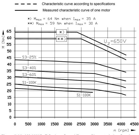
Figure 7-35, AM 1550D–E Series - Speed-Torque Characteristics Graph
