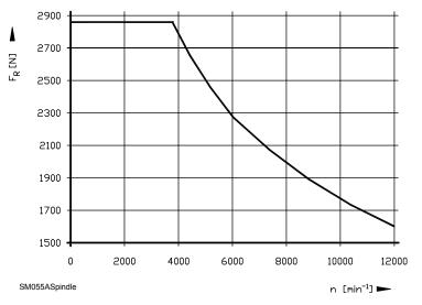
Figure 7-92, SM 055D, SM 055F, SM 075D, SM 075F, SM 100D, SM 100F - with Spindle Bearing - Permissible Axial Force on the Motor Shaft
