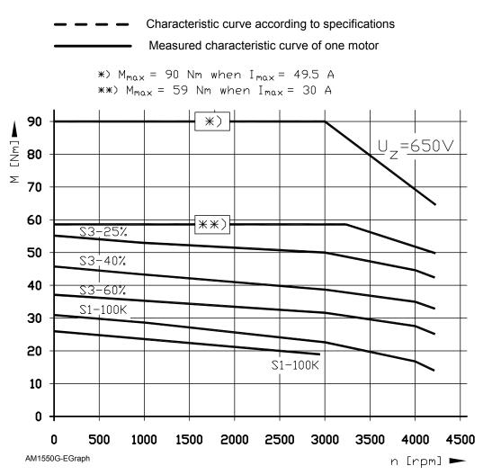
Figure 7-36, AM 1550G–E Series - Speed-Torque Characteristics Graph
