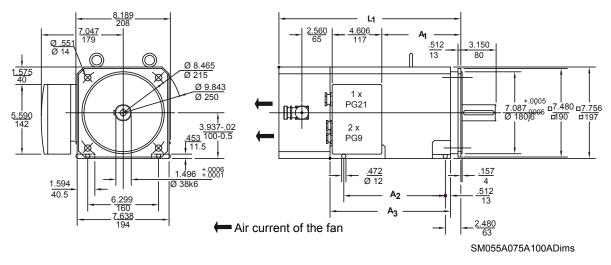
Figure 7-69, SM 055A, SM 075A, SM 100A - Dimensional Drawing
