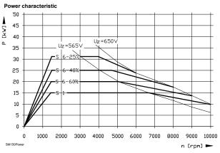
Figure 7-63, SM 150C-F - Power Characteristics Graph
