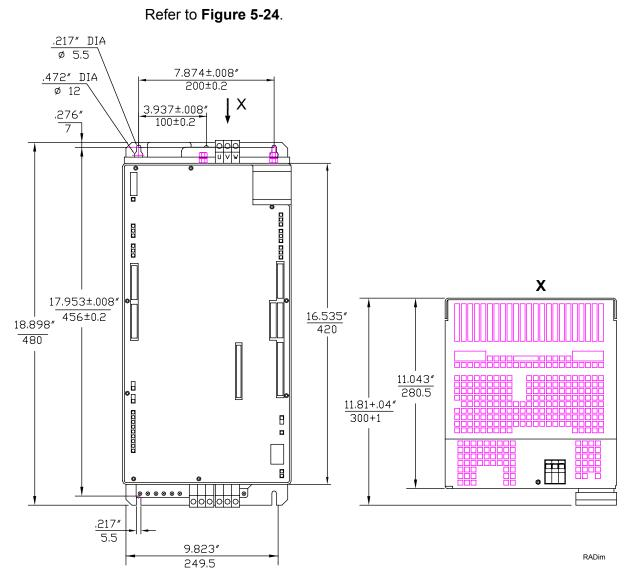
Figure 5-24, RA 201A, RA 301C, RA 411C Amplifier Dimensions
