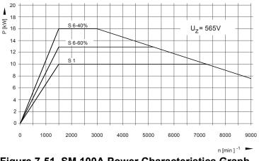
Figure 7-51, SM 100A Power Characteristics Graph
