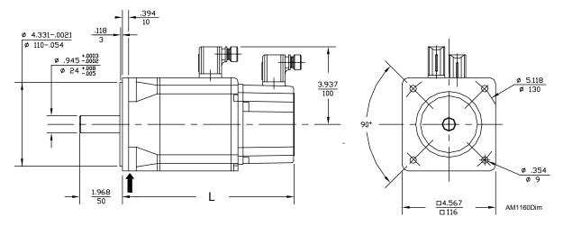
Figure 7-41, AM 1160 Series - Dimensional Drawing
