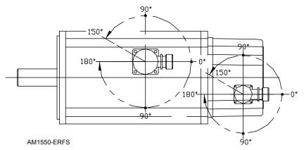
Figure 7-19, AM 1550E Series Rotatable Flange Socket
