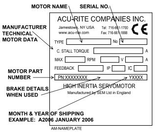
Figure 7-1, Axis Motor Nameplate
