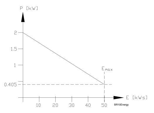
Figure 3-3, BR 10F - Braking Performance Function of Braking Energy
