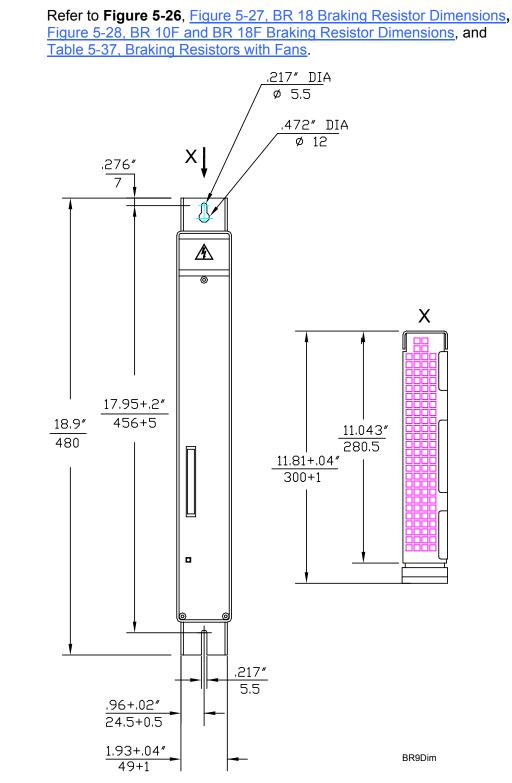
Figure 5-26, BR 9 Braking Resistor Dimensions
