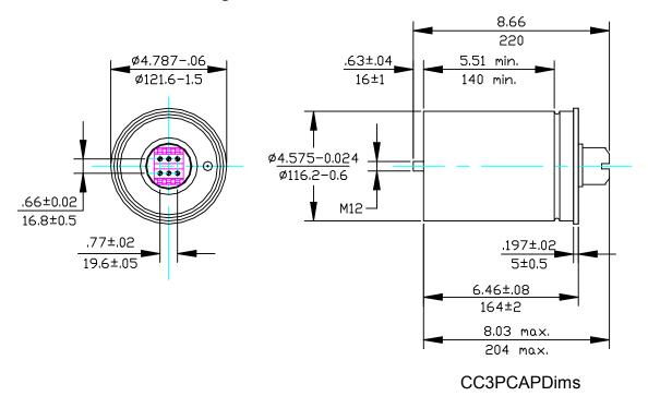
Figure 6-33, Three-Phase Current Capacitor, CC 3P, Dimensions
