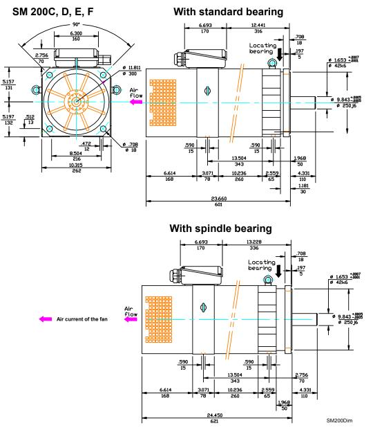
Figure 7-76, SM 200C–F - Dimensional Drawing
