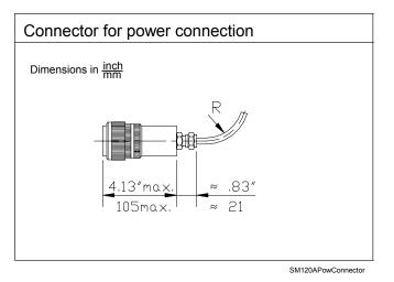
Figure 7-72, SM 120A - Connector for Power Connection
