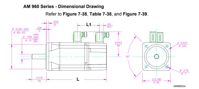
Figure 7-38, AM 960A and AM 960AB - Dimensional Drawing
