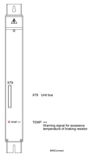
Figure 5-13, BR 9 Braking Resistor
