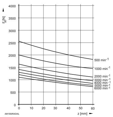
Figure 7-83, AM 1550 Series - Permissible Radial Force on the Motor Shaft (F<sub>R</sub>)
