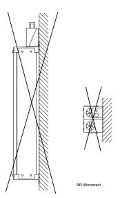
Figure 4-5, BR 18 - Incorrect Installation
