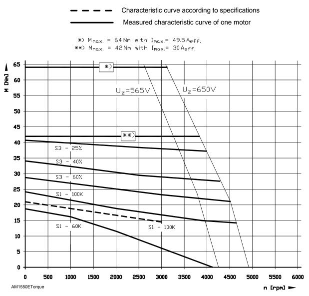
Figure 7-31, AM 1550E Series - Speed-Torque Characteristics Graph
