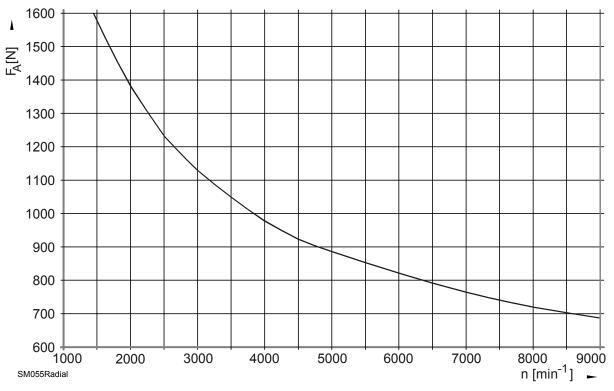
Figure 7-89, SM 055A, SM 075A, and SM 100A - Permissible Radial Force on the Motor Shaft
