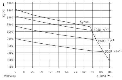
Figure 7-97, SM 120C, SM 120E, SM 150C, SM 150E, SM 200C, SM 200E, SM 240C, SM 240E - with Standard Bearing - Permissible Radial Force on the Motor Shaft
