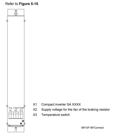
Figure 5-15, BR 10F and BR 18F Braking Resistors
