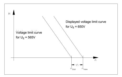
Figure 7-3, Characteristic Curves for Axis Motors
