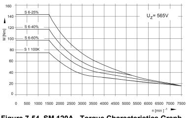
Figure 7-54, SM 120A - Torque Characteristics Graph
