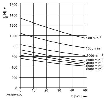
Figure 7-81, AM 1160 Series - Permissible Radial Force on the Motor Shaft (F<sub>R</sub>)
