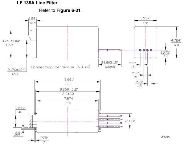
Figure 6-31, LF 135A Line Filter, Dimensions
