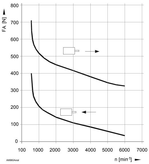
Figure 7-79, AM 960A, AM 960AB - Maximum Permissible Axial Force (F<sub>A</sub>)
