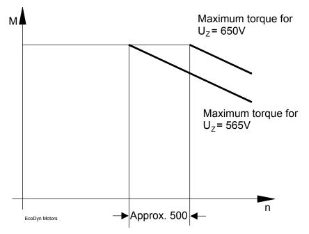
Figure 7-4, Characteristic Curves for Axis EcoDyn Motors
