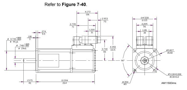
Figure 7-40, AM 1150 Series - Dimensional Drawing
