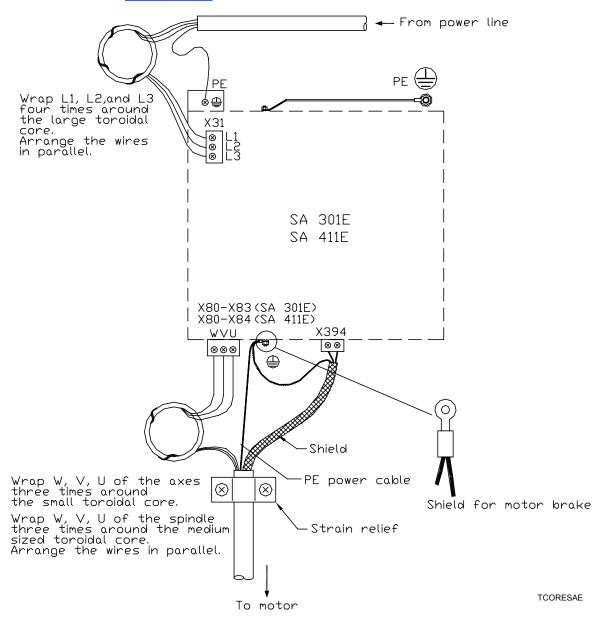
Figure 5-20, SA 301E, SA 411E Toroidal Core Configuration
