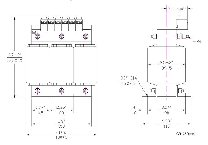
Figure 6-29, CR 135 Commutating Reactor, Dimensions
