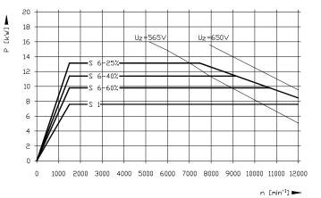
Figure 7-57, SM 075C-F - Power Characteristics Graph
