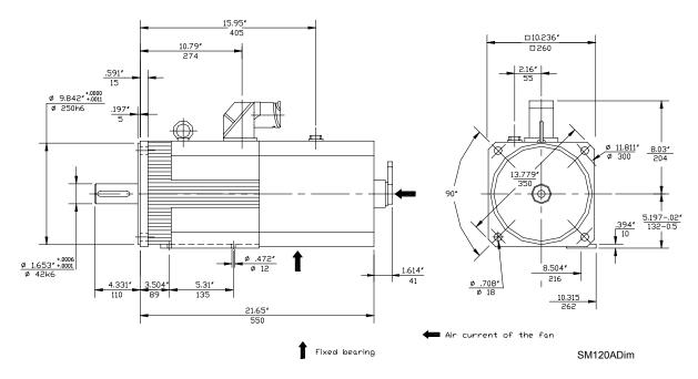
Figure 7-71, SM 120A - Dimensional Drawing
