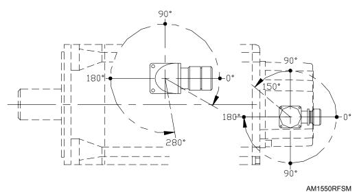
Figure 7-17, AM 1550 Series (starting in mid-2002) Rotatable Flange Socket
