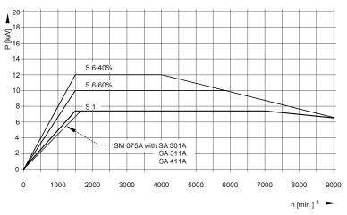
Figure 7-49, SM 075A Power Characteristics Graph
